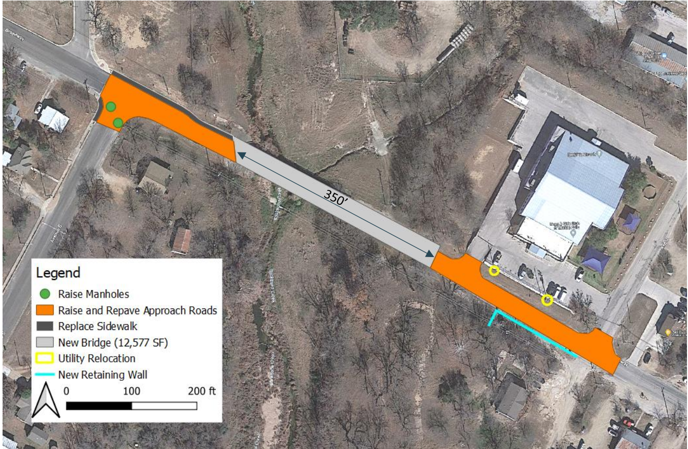
Figure 4: Proposed Bridge Improvements
