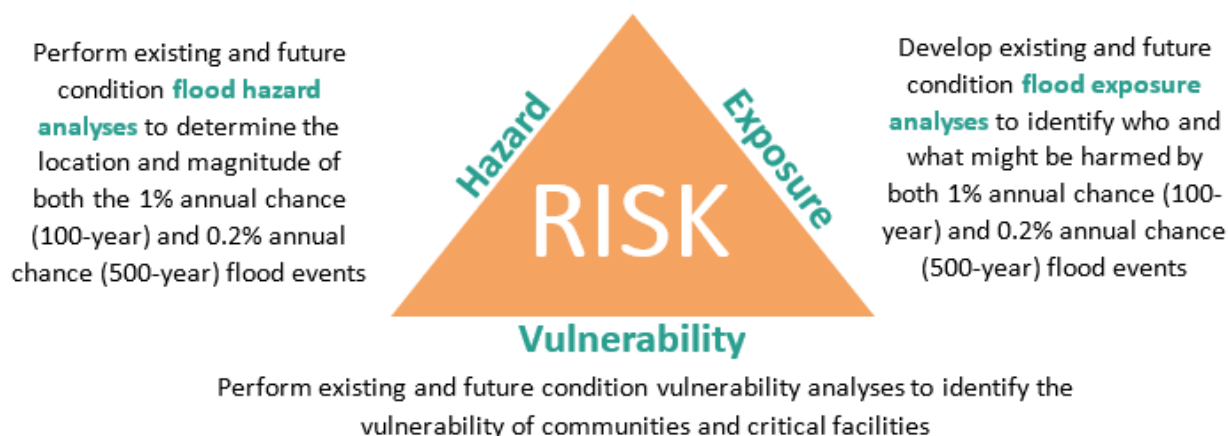
Figure 2.1 TWDB Flood Risk Analyses Triangle Framework
