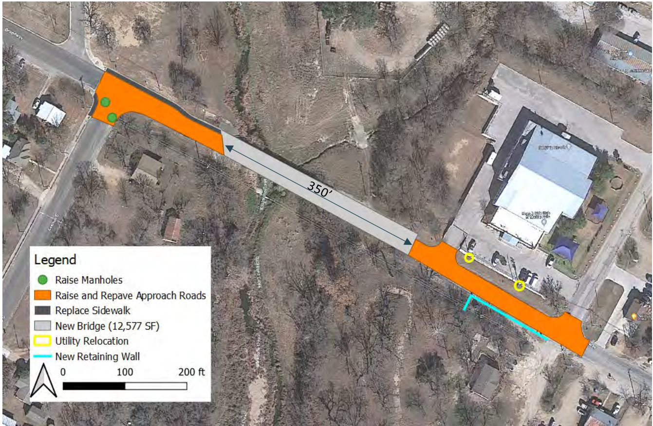
Figure 4: Proposed Bridge Improvements
